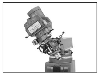
Figure 21. Head rotated to the left.
